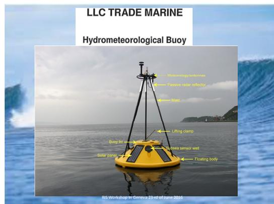
Fig.4. Hydrometeorological buoy
